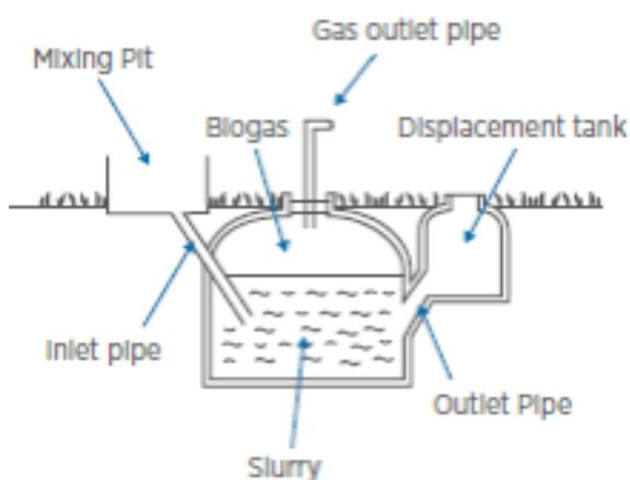
Figure 17. Fixed Dome Digester Diagram
