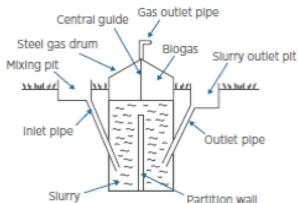
**Figure 21. Diagram of a Floating Drum System**
