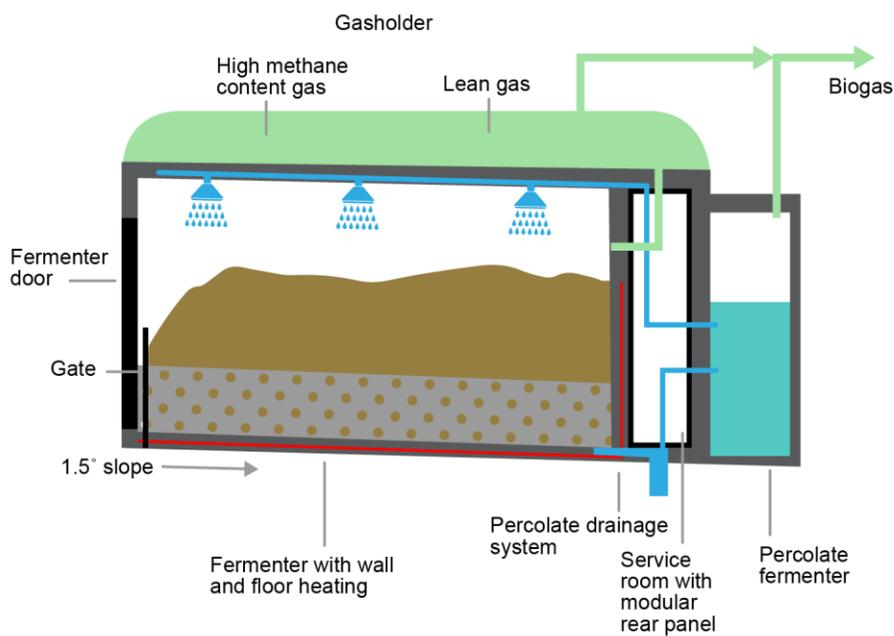
**Figure 30. Diagram of a Dry AD System**
